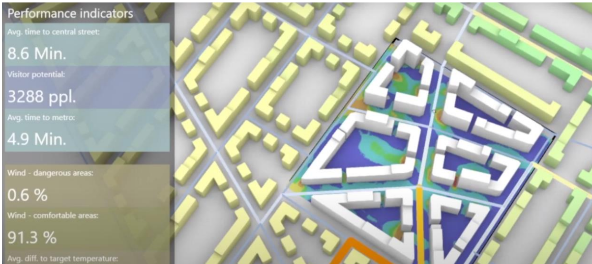
Figure 3: The web interface of InFraReD computes performance indicators for urban analysis (InFraReD tutorial, 2021).
