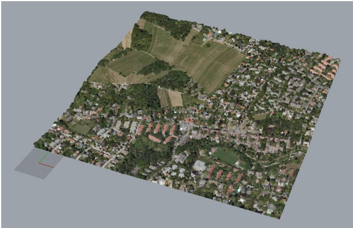
Fig. 4: 3D data of the site in the form of a point cloud is available for the Rhinoceros environment.
