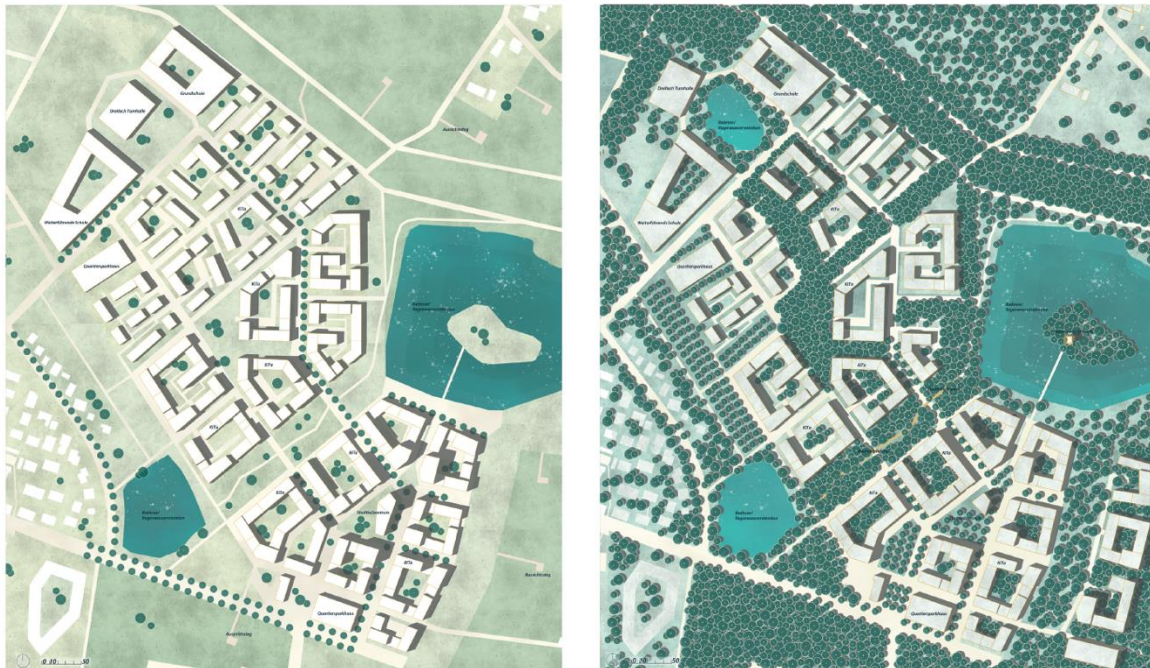
Figure 6.4.4-1: Comparison of urban design variants. Left developed for heat-loving insect species, right for forest-dwelling birds and mammals. (Design and illustration: D. Höhnel)
